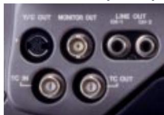
EBU TC I/O connectors for multi-camera shooting allow synchronisation to other devices such as Nagra, DAT's and TC Slate. The GY-DV700WE's internal EBU TC reader generator provides user bit at any tape speed.
